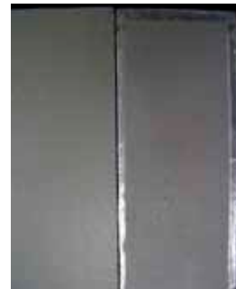
Above left: Shakespeare composite specimens approaching 15000 hours of QUV exposure testing (the background) and unexposed control. Most of the color difference is caused by the fact that the tested sample is wet, and the comparison control is dry.
