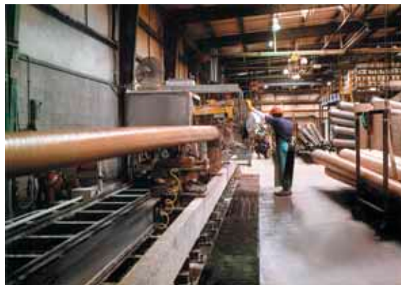
Below right: Polishing operation for a Shakespeare smooth composite pole. These poles, as well as veil finish (un-sanded) receive an additional non-woven, resin-soaked winding that further extends UV life.
